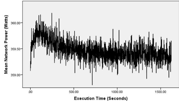
Fig. 9. Power usage of four network related domains collected from profiling code. Displays increasing then decreasing power curve at beginning of execution leveling out around 500 seconds. Stays within 1 W of starting value.
