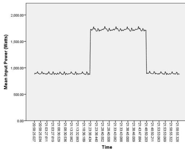
Fig. 7. Power usage as collected from the environmental database for the BPMs. Sharp increase/decrease shows point in time when application switches from stopped to running and back to stopped.
