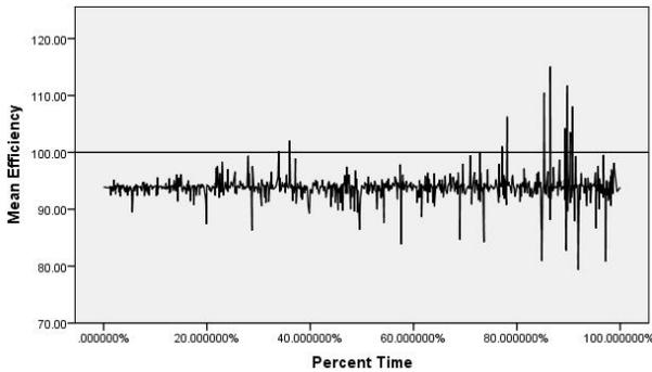
Fig. 5. AC/DC conversion efficiency of BPMs over time. As expected, the efficiency remains relatively constant over the course of execution for a given job. Because the sensors on the BPM are not designed for instantaneous readings, attempting to determine instantaneous efficiency readings is unrealistic and therefore results in incorrect values (i.e., over 100%). However, when looked at over a long period of time, it can be deduced that the BPMs maintain about 94% conversion efficiency.
