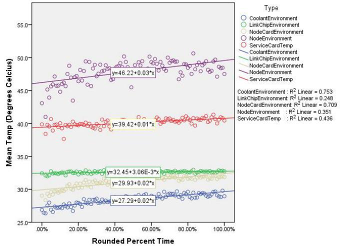
Fig. 6. Temperature fluctuation as a function of time. As expected, the system gets “hotter” as jobs run. Most sensors indicate a 2 to 3 degree increase of individual components. Bootup and shutdown times not taken into consideration because of fluctuation in those times, thus it is expected the temperature increase would be more dramatic than depicted.
