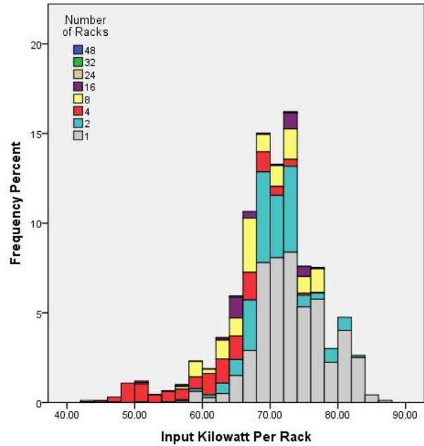
Fig. 3. Frequency distribution of average per-rack power consumption. Figure indicates most jobs fall into the 60-80 kW bins and all jobs are between 40 and 90 kW.
