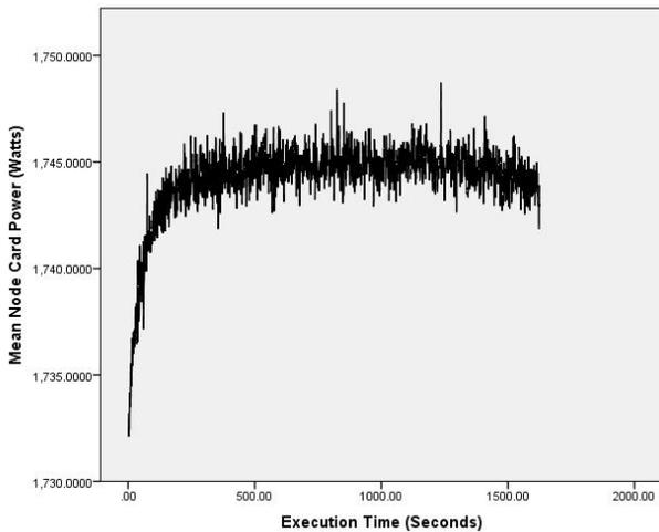
Fig. 8. Power usage of node card collected from profiling code. Because the EMON API allows for much faster sampling, the increase in power consumption when the job actually runs is not as dramatic as the figure from the BPM.
