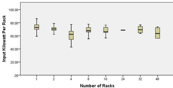
Fig. 2. Boxplot of kilowatt usage per rack. Shows no significant difference in jobs running on small or large number of racks. Average power consumption is 70.32 kW per rack.
