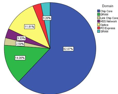
Fig. 10. Pie chart showing relative percentages of total power usage consumed by each of the 7 power domains. Intense network activity largely contributing to optics percentage.
