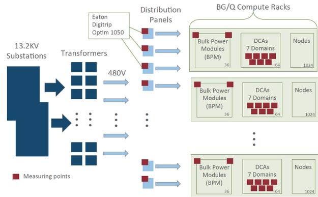
Fig. 1. Mira 480V compute power distribution system.
