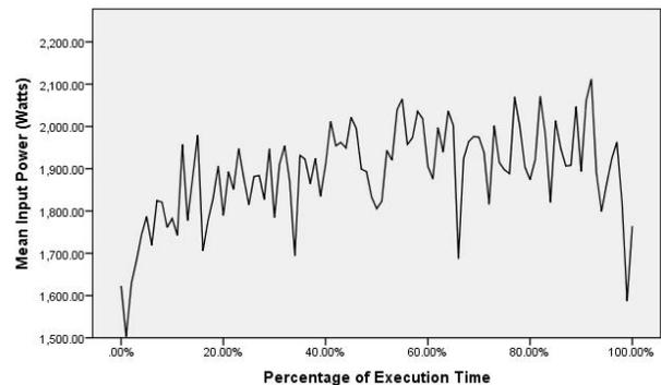
Fig. 4. Average power usage profile of a job running on system. Shows power on average does increase as a function of time. First and last 5% likely influenced by startup and shutdown times.
